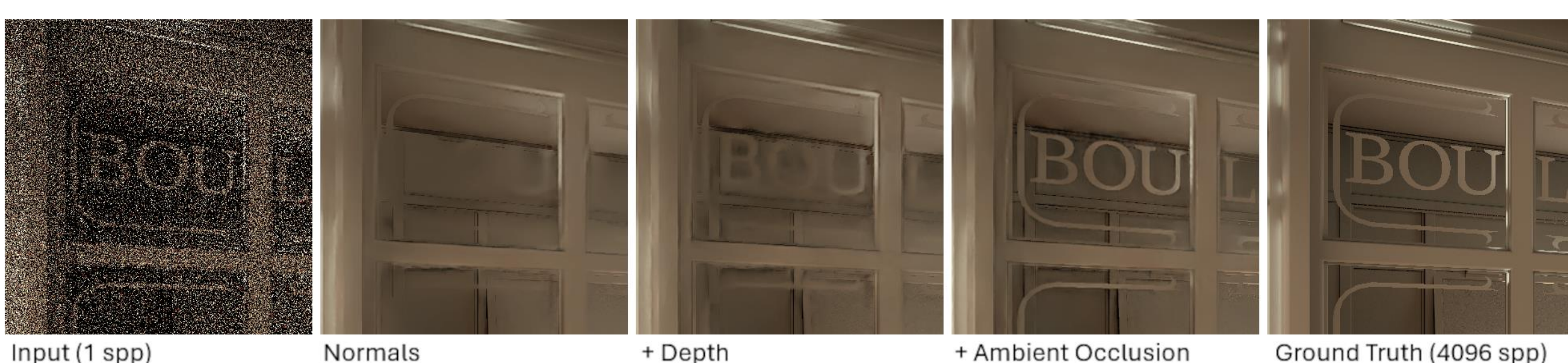
Figure 3: Ambient occlusion helps the filter restore the lost structural information while also improving the quality of denoised shadows.
